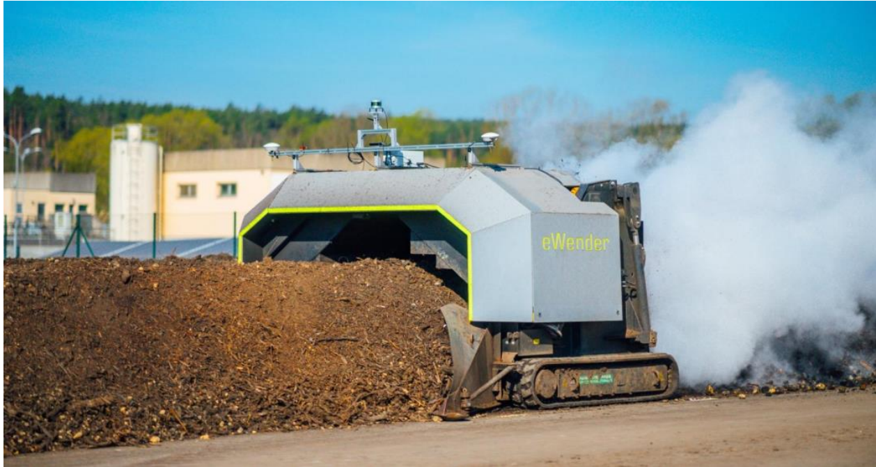
Autonomous and electric compost turner, Source: Futurezone (2023)
