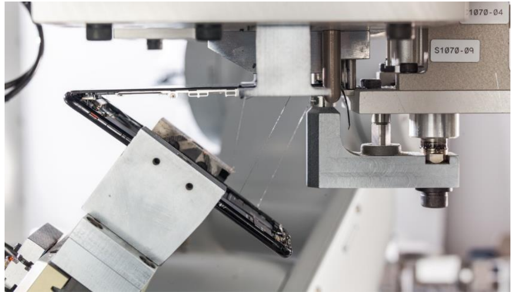
Apple's recycling robot "Daisy", Source: Apple (2018)
